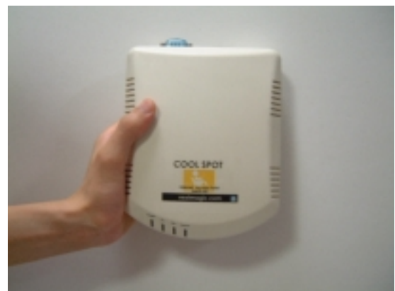
Photograph: Wireless LAN router for COOLSPOT (Model: NAPS-02 ) A5 size and 480g weight. (included PHS card's weight)
